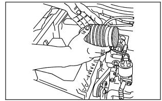
5. Remove the air outlet duct.
